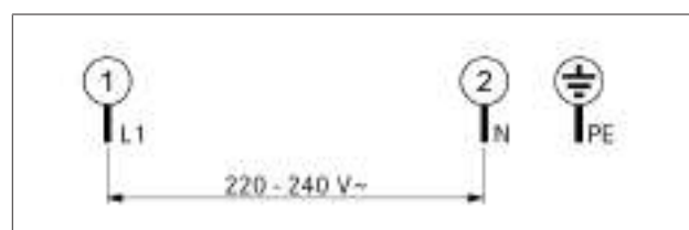
Fig. 4.86 1-phase connection diagram
